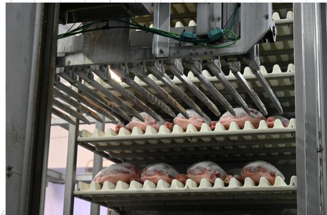
Robot for loading/unloading operations of the hams from the chassis. with simultaneous loading of two or more hams.
